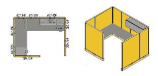
Per Station: (1) BBF Pedestal, (1) FF Pedestal, (1) 48" Flipper Unit with Tasklight
